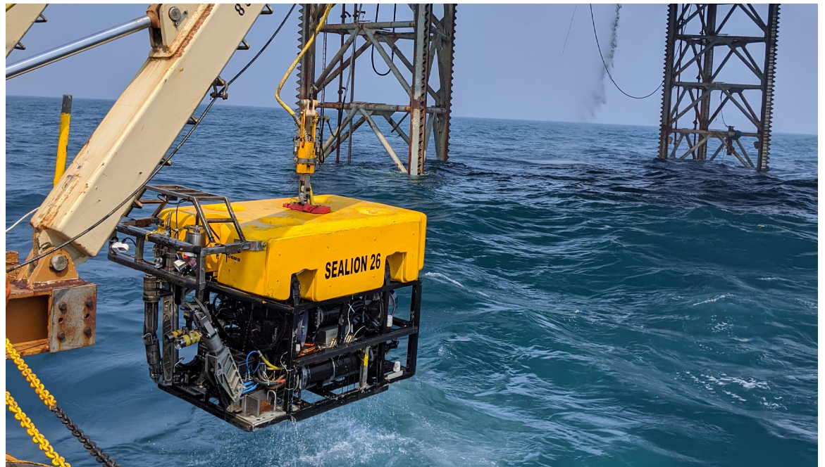
Remote Operated Vehicle used during B-80 drilling Campaign
